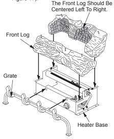
Figure 17 - Installing Grate and Logs
